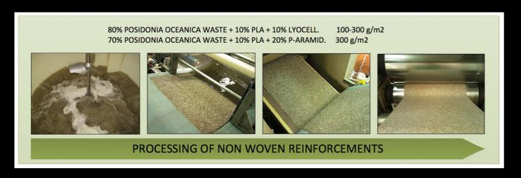
The wet-laid non-wovens have been used as reinforcement in thermoplastic and thermo-stable composites assessing their applicability in the following composite manufacturing processes: thermos-compression moulding, resin infusion (VARTM) and manual laminating (HAND LAY-UP and VACUUM BAG). We have developed a high variety of composite materials in the context of this project.
